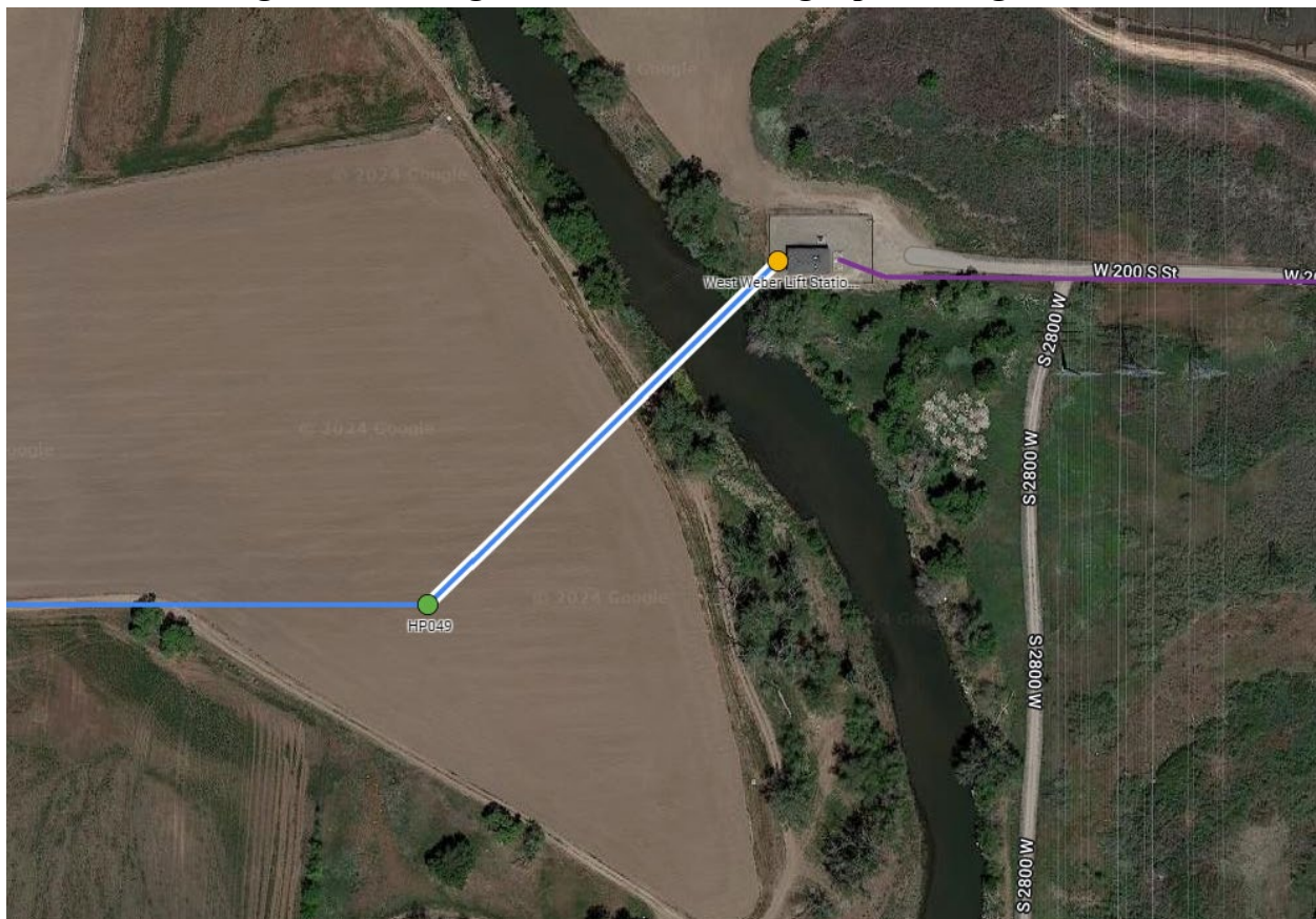
Figure 1: Existing Weber River Crossing Pipeline Alignment
